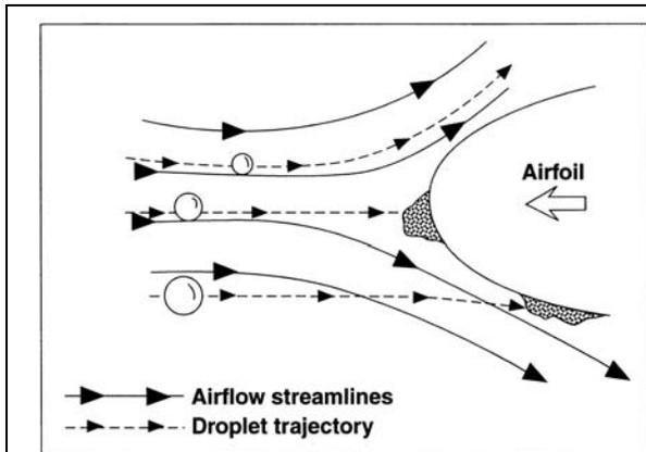
**Figure 6** – Airflow around a typical airfoil. Also shown are possible droplet trajectories. (From Perkins and Reike, 2001)
