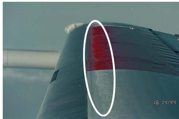
**Figure 7** – Picture of icing runback beyond the protected surface (circled). Icing encounter occurred on February 16, 2000 during AIRS and was classified by the pilots as severe. (From Isaac et al, 2001)
